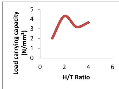
Fig. 9: Wall Panel Load Carrying Capacity V/S H/T Ratio Plot
