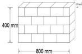
Fig. 1: Details of Panel Specimen
