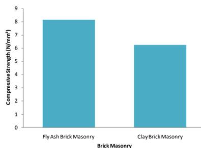
Fig. 8: Comparison Of Compressive Strength Of Fly Ash Brick Masonry And Clay Brick Masonry
