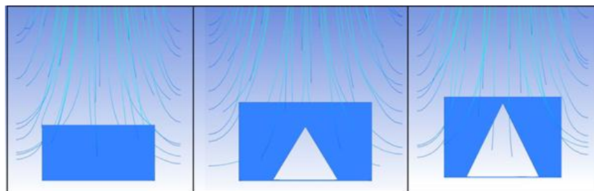
Fig. 6: Velocity Contours for Fin without Notch and Fin with 20% and 40% Notch
