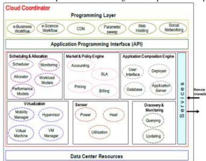
Fig. 2: Cloud Coordinator Software Architecture
