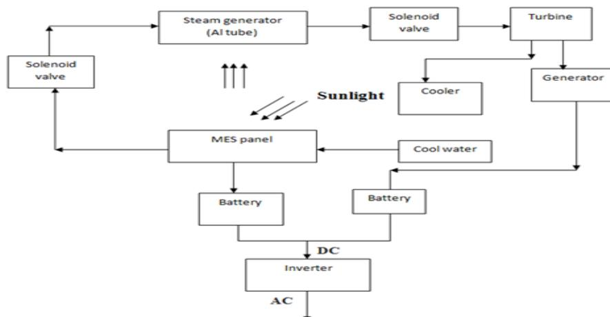
Fig. 1: block diagram of MES energy system
