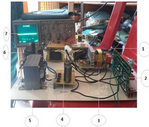
Fig. 6: Hardware Structure of ZSI Fed BLDC Motor
