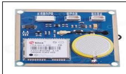
Fig. 3: GPS Module Consisting of U-Blox LEA 6-H
