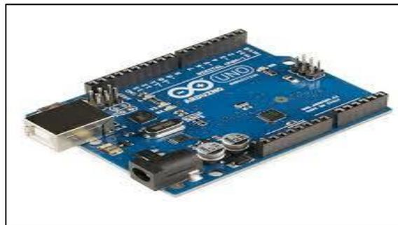
Fig. 7: Arduino Uno Microcontroller
