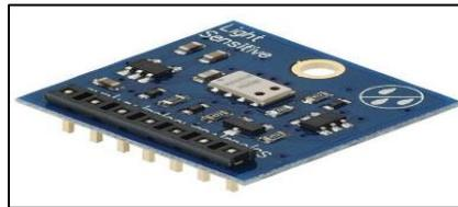
Fig. 2: Parallax MS-5607 Altimeter Module
