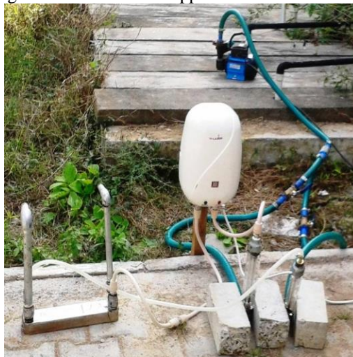
Fig. 3: Actual Experimental Setup of Brazed Chevron Type Plate Heat Exchanger
