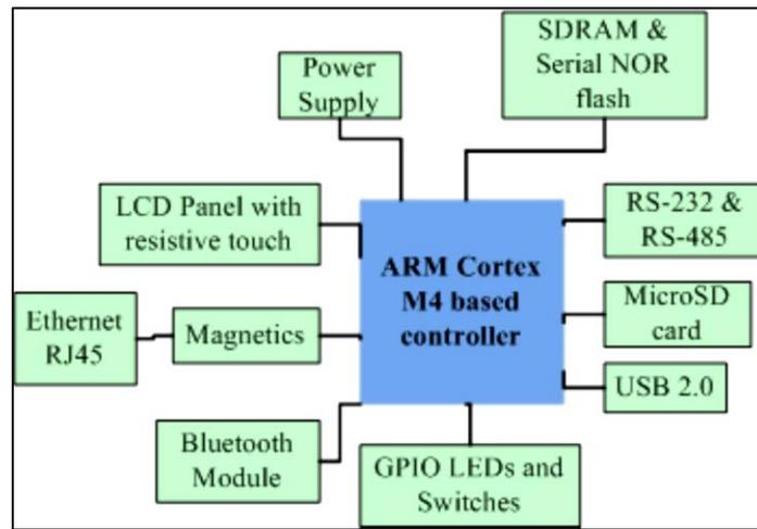
Fig. 1: Block Diagram of HMI Panel
