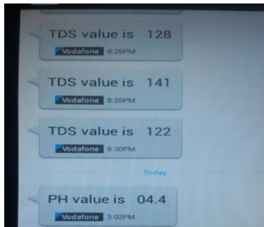
Fig. 7: SMS from GSM When Threshold Exceeded
