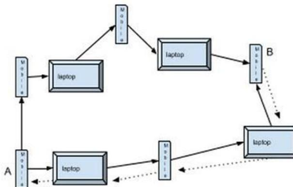
Fig. 1: RREQ and RREP messages in MANET using AODV
