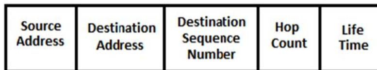
Fig. 4: Route Reply Frame Format
