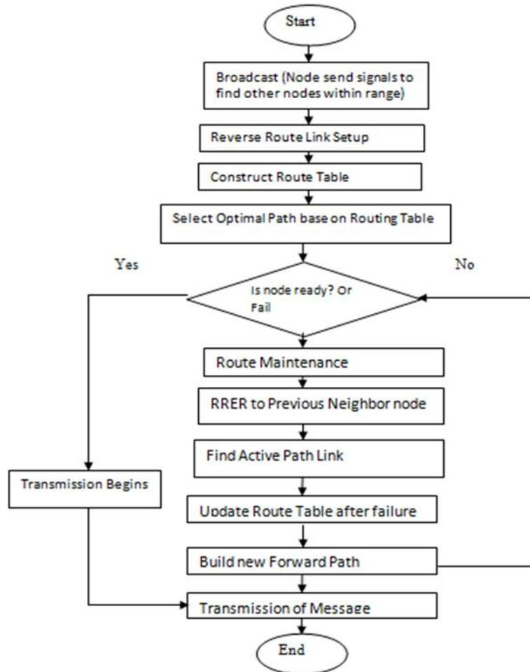
Fig. 6: Work Flow of Implementation Methodology
