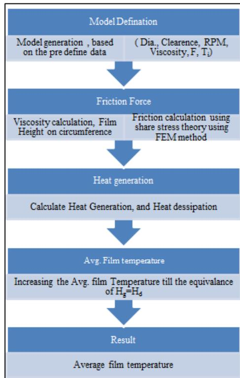
Fig. 3: Algorithms Adopted For Calculating Average Oil Film Temperature
