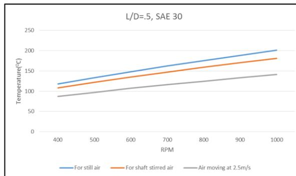
Fig. 11: Temperature Variation on Changing RPM at L/D Ratio 0.5 at Three Different Conditions
