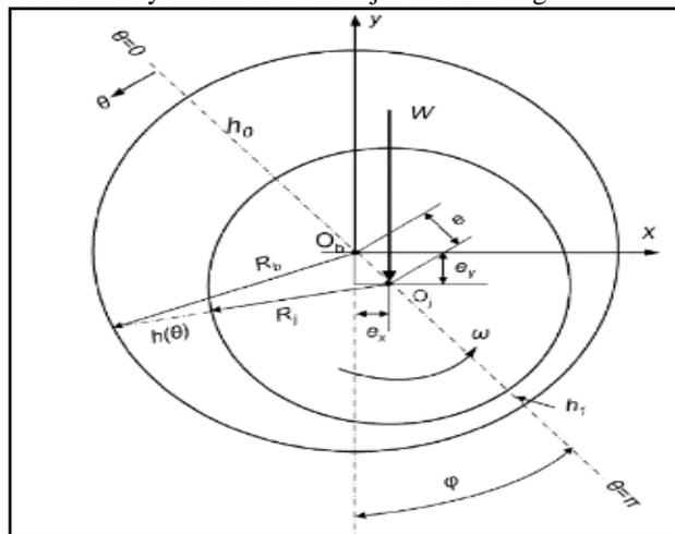
Fig. 1: Schematic Diagram of Journal Bearing
