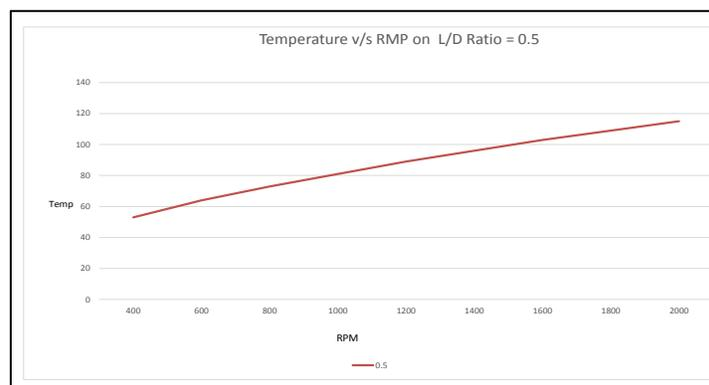
Fig. 8: Temperature Variation on Changing RPM at L/D Ratio 0.5
