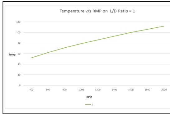
Fig. 9: Temperature Variation on Changing RPM at L/D ratio 1
