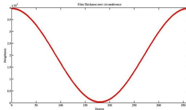
Fig. 4: Film Thickness Variation across Periphery
