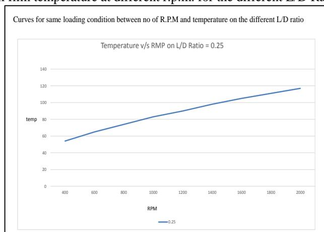
Fig. 7: Temperature Variation on Changing RPM at L/D ratio 0.25
