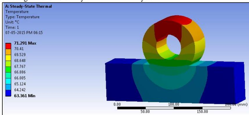
Fig. 5: Temperature variation across the bearing using ANSYS
