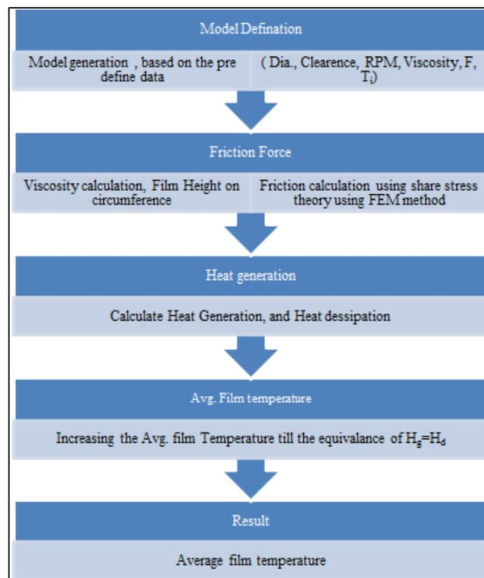
Fig. 1: Algorithms Adopted For Calculating Average Oil Film Temperature
