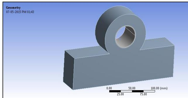
Fig. 2: Model Generation of Bush Type Journal Bearing
