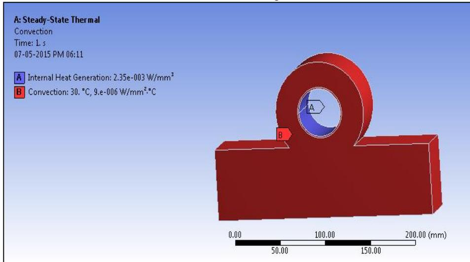
Fig. 4: Applying Boundary Conditions on the Element in ANSYS
