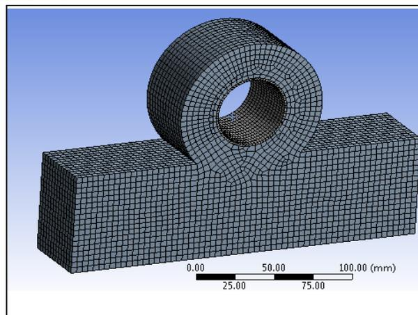
Fig. 3: Hexagonal Element Meshing of Model in ANSYS
