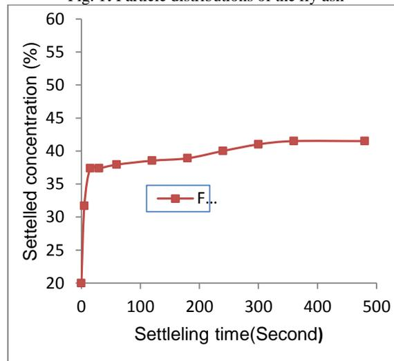
Fig. 2: Settled concentration of fly ash
