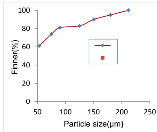
Fig. 1: Particle distributions of the fly ash
