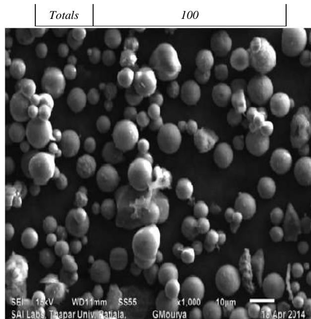
Fig. 3: SEM of Rolling mill ash Sample
