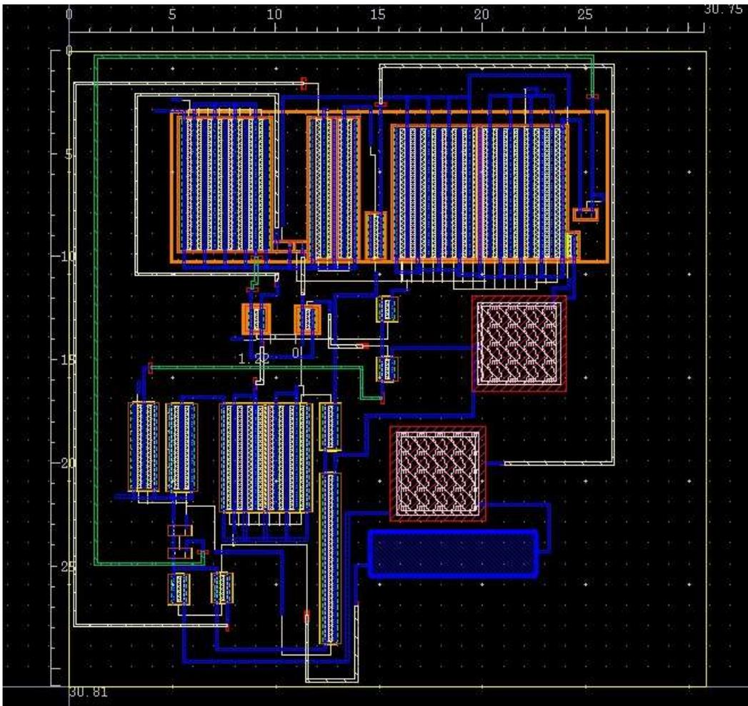
Figure 11 : Physical layout of rail-to-rail op-amp
