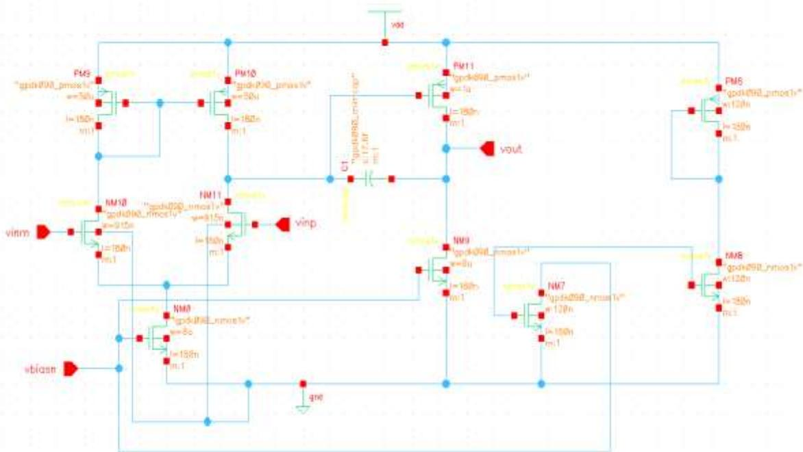
Figure 6 : NMOS differential pair schematic
