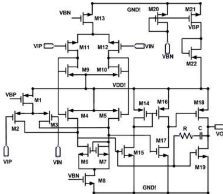
Figure 3 : Rail-to-rail operational amplifier [2]
