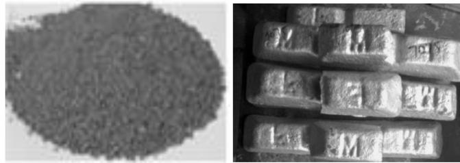
Fig. 1: Bottom Ash and Al7075 ingot
