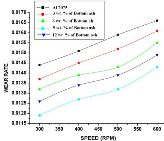
Fig. 12: Effect of wear rate at varying speed
