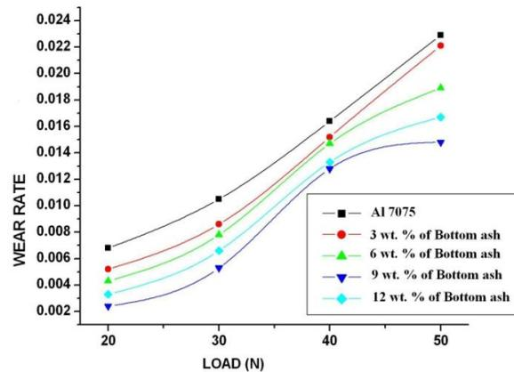
Fig. 13: Effect of wear rate at varying load
