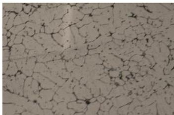
Fig. 7: Microstructure of pure Al 7075
