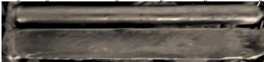
Fig 4 Cast Rod and and Slab of Aluminium Matrix Composite
