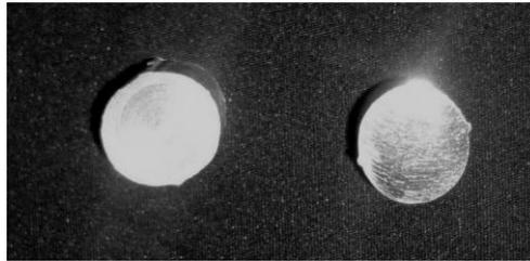
Fig 5 Polished specimen used for microstructure
