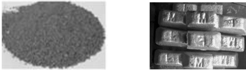
Fig 1: Bottom Ash and Al 7075 ingot
