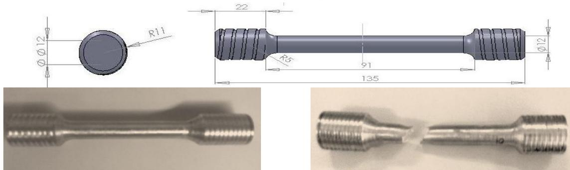
Fig 6 Tensile Test Specimen before and after testing
