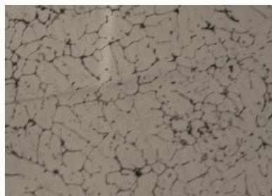
Fig. 7: Microstructure of pure Al 7075
