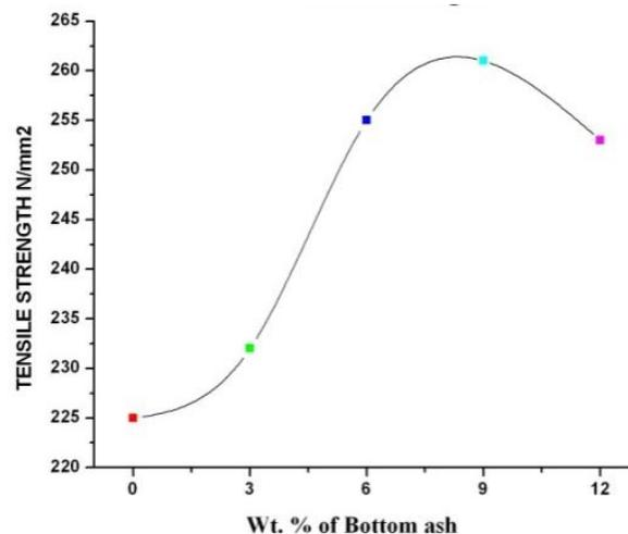
Fig. 12: Variation of tensile strength with the weight fraction of bottom ash
