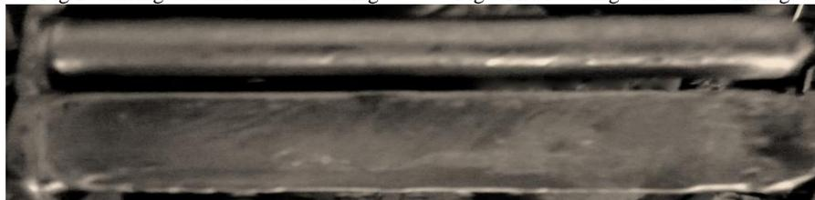
Fig 4: Cast Rod and and Slab of Aluminium Matrix Composite
