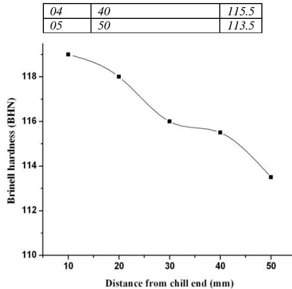
Fig 15: BHN v/s Distance from chill end
