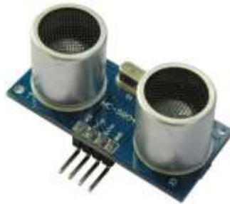
Fig. 6: Ultrasonic sensor
