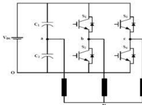
Fig. 1: Four Switch Three Phase Inverter.
