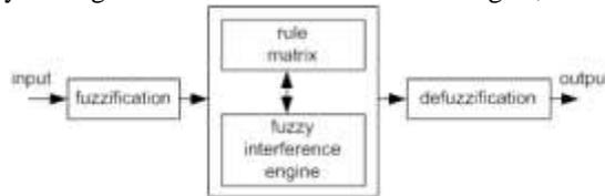
Fig. 6: Basic Fuzzy logic controller
