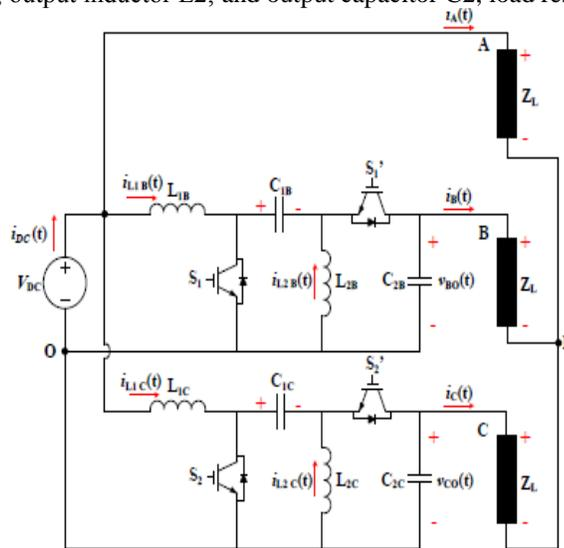
Fig. 2: FSTP SEPIC Inverter
