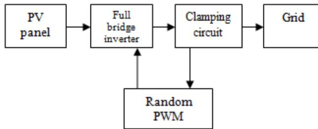
Fig. 4: Block diagram representation of RPWM methodology.
