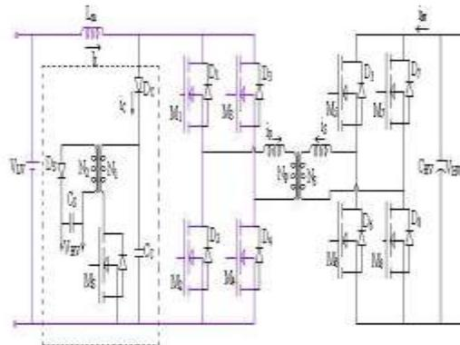
Fig. 2: Mode 1 ( $M1-M4$  ON and  $L_m$  charged)
