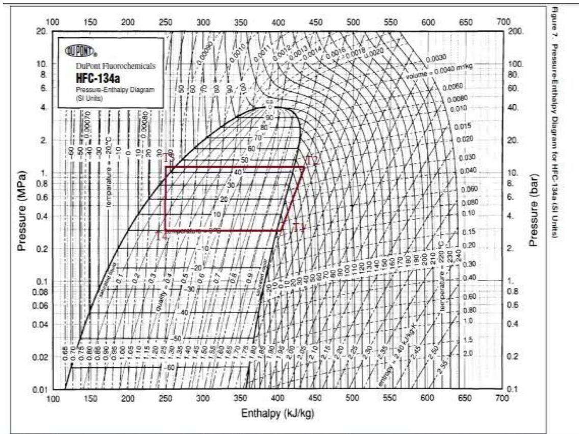
Fig. 5.1: R-134a representing the Sub-Cooling Process after Condensation.
