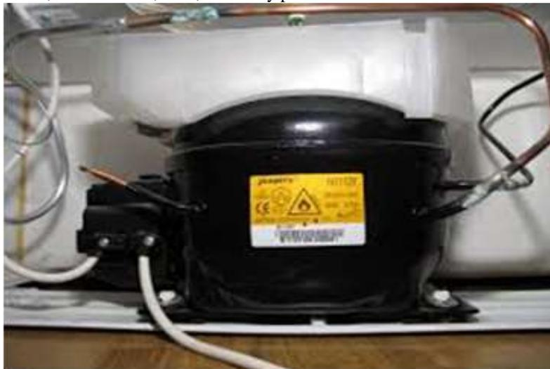
Fig. 2.1: Hermetic sealed compressor
