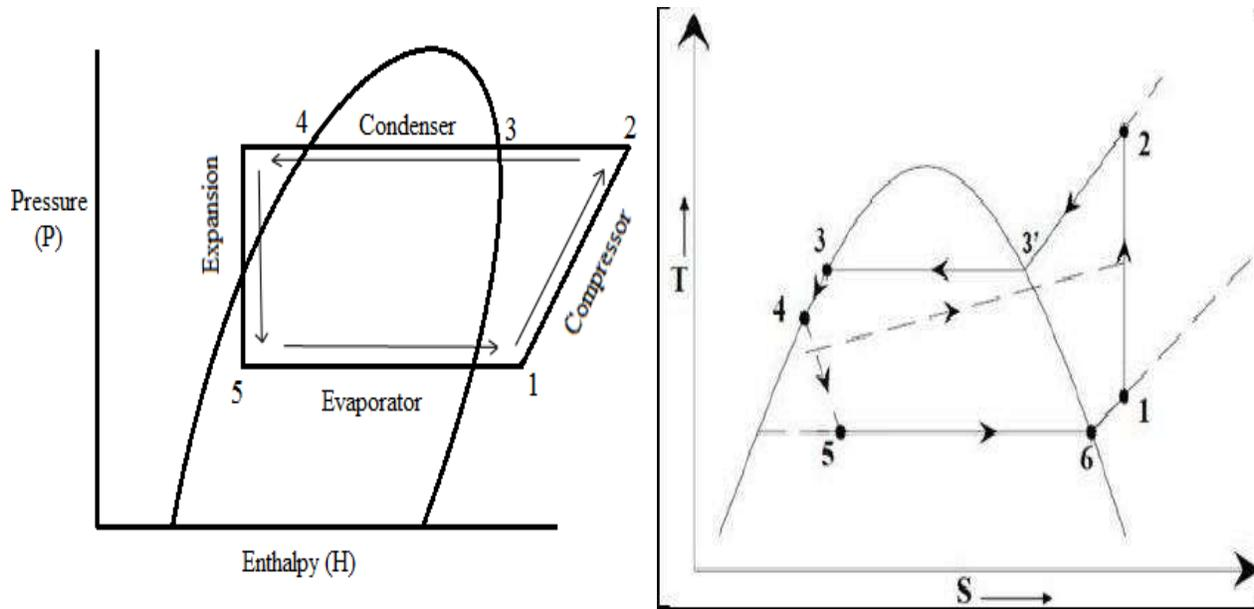
Fig. 3.1: P-H and T-S diagram simple vapour compression refrigeration cycle.
