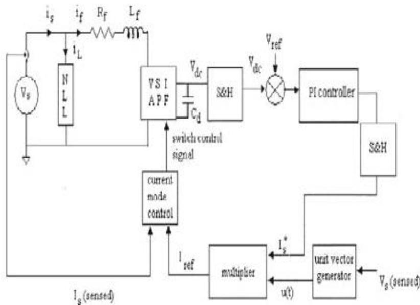
Fig 2: Block diagram of PI based APF
