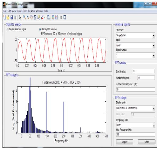
Fig 8: FFT Analysis of source current (Using PI controller)
