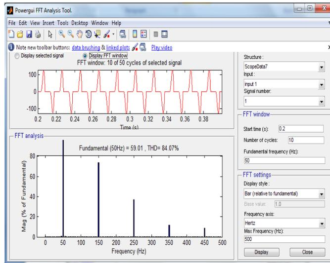
Fig 7: FFT Analysis of source current (Conventional power circuit)
