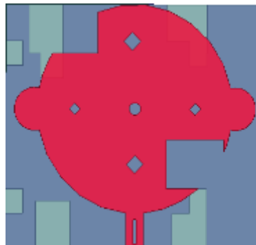
Fig. 5: Slotted patch of the design 2
