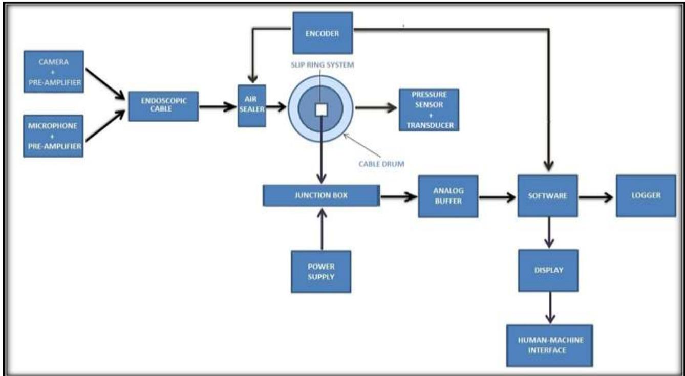
Fig. 1: Block Diagram representation of the proposed detector.
