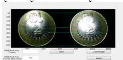
Fig. 4: Coin feature extraction using SIFT.
