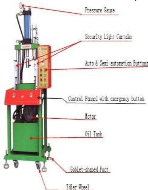
Fig. 3.1: Structure of hydraulic machine
