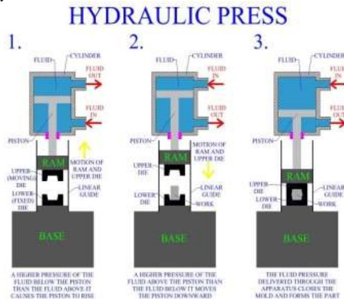
Fig. 3.2: Stages of hydraulic press
