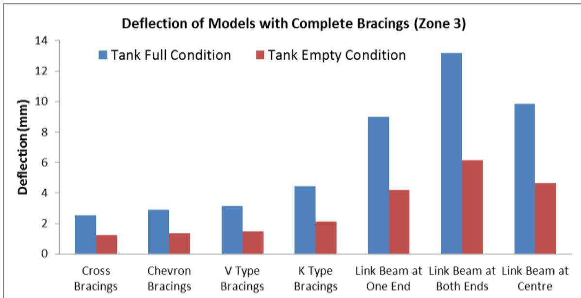
Fig. 1: Deflection of Models with Complete Bracings (Zone 3)
