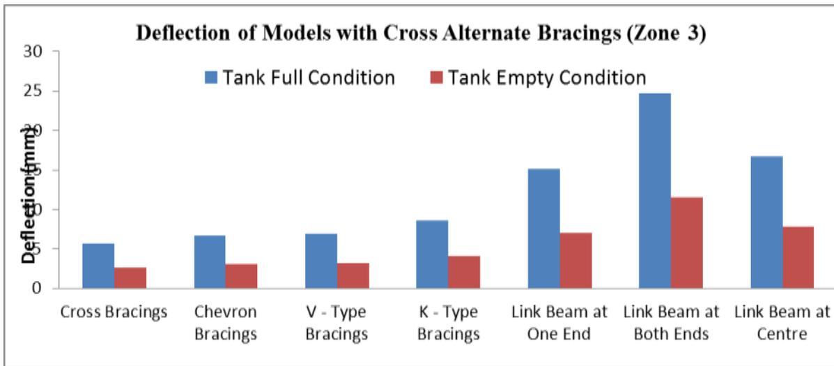
Fig. 3: Deflection of Models with Alternate Cross Bracings (Zone 3)
