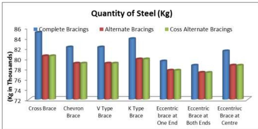
Fig. 6: Quantity of Steel (Kg)
