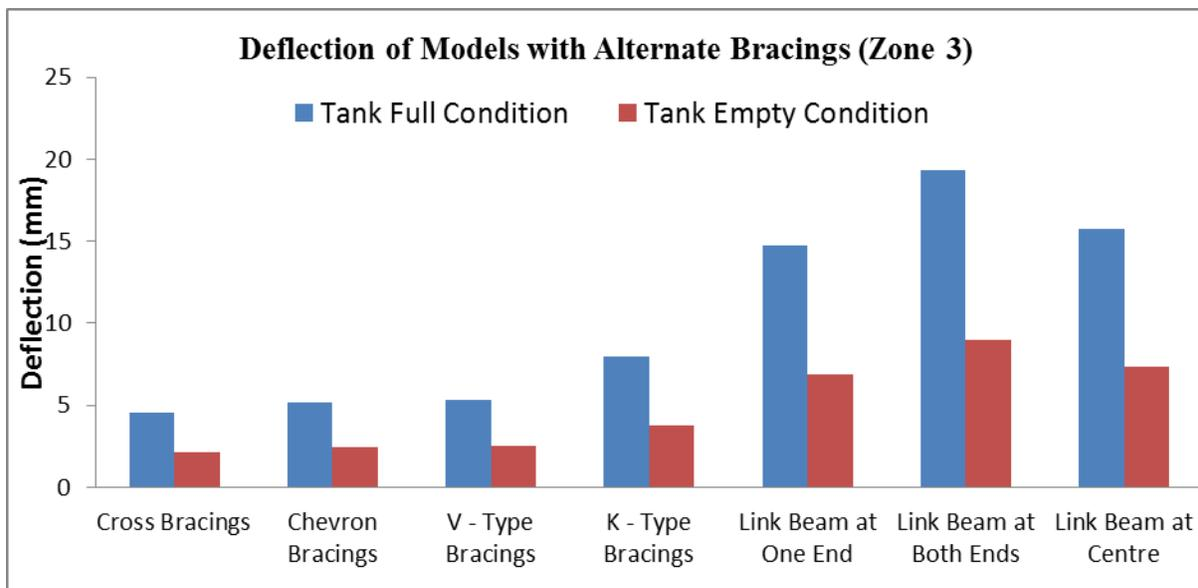
Fig. 2: Deflection of Models with Alternate Bracings (Zone 3)
