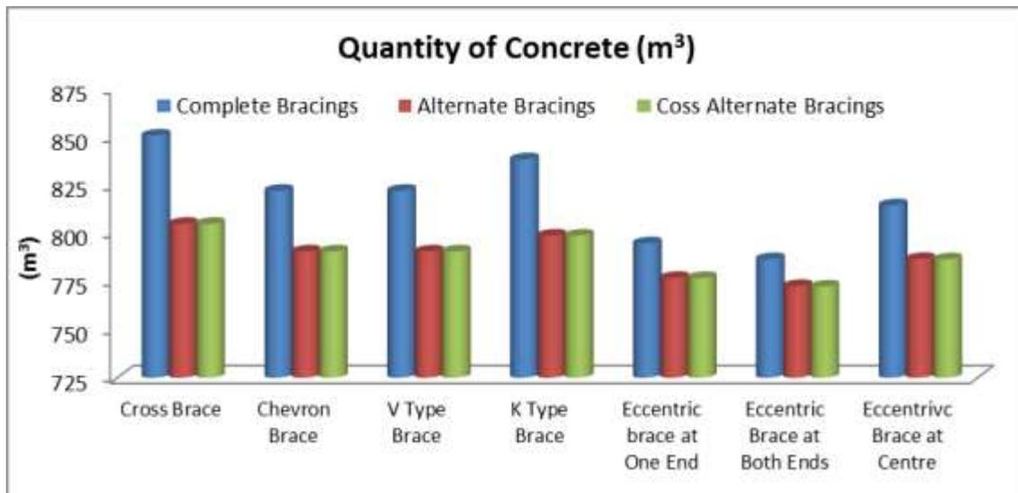
Fig. 5: Quantity of Concrete (m3)
