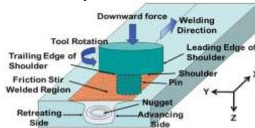
Fig. 1: Process principles for friction stir welding [5].
