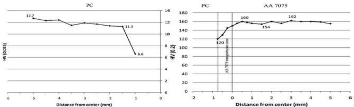
Fig. 5: Vickers micro hardness at PC joint interface and at AA7075 base material and AA 7075 transportation interface. [9]
