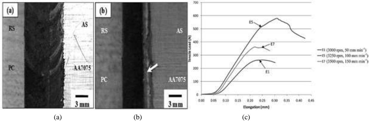
Fig. 4: Surface appearances of the welded joint at 3500 rpm and 50 mm min<sup>-1</sup> (a) front side (b) rear side (c) Tensile load curve for highest, middle, and lowest load. [9]
