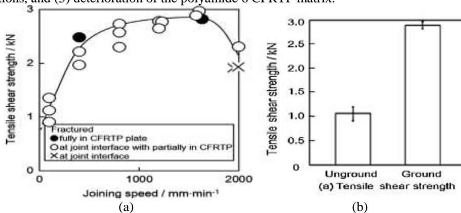
Fig. 2: (a) The relationship between joining speed during FLJ and the tensile shear strength of the joints (b) Tensile shear strength of the unground- and ground-A5052/CFRTP joints [7].
