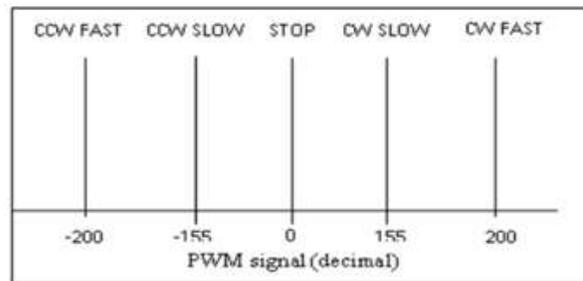
Fig. 4(b): The fuzzy output set (DC motor speed)
