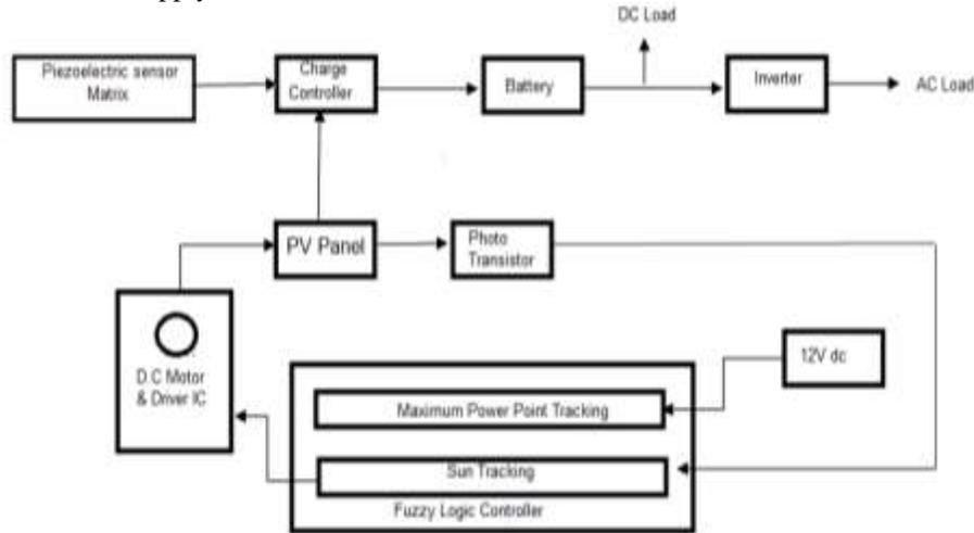
Fig. 1: Block Diagram of implemented System.
