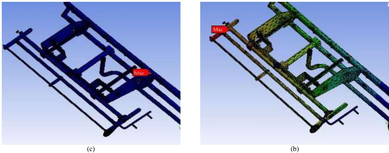
Fig. 7: Numerical analysis of spray coater arm
