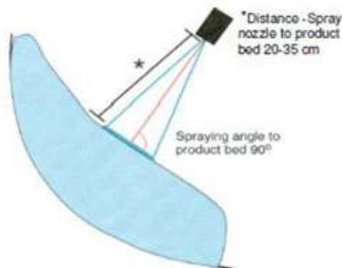
Fig. 5: Representation of desired spray gun to bed distance and angle of spray gun to tablet bed
