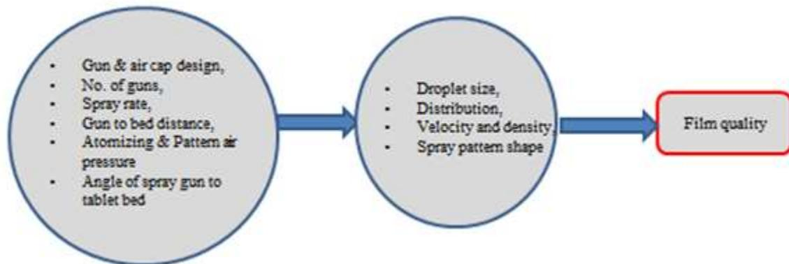
Fig. 3: Factors to be considered while designing a Spraying system
