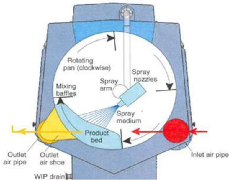
Fig. 1: Schematic diagram representing functional principle of pan coater [1]
