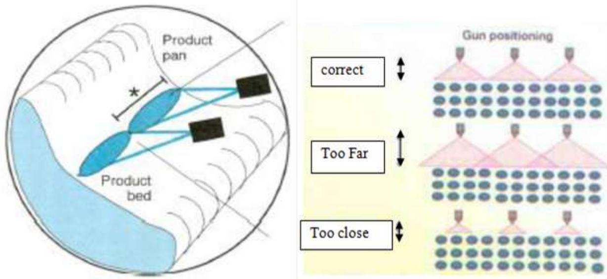
Fig. 4: Representation of elliptical shape of spray pattern in order to achieve uniform coating
