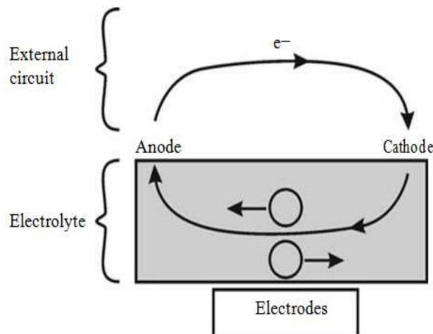
Fig. 2: An electrode, a circuit for a cell which is converting chemical energy to electrical energy. The motion of negative charges is clockwise and forms a closed loop through external wires and load and the electrolyte in the cell.
