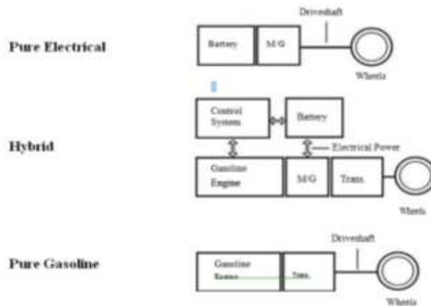
Fig. 1: Components of a hybrid Vehicle that combines a pure gasoline with a pure EV.
