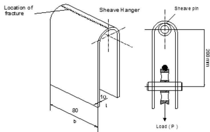
Fig. 2: The crane sheave hanger (Enlarge View)
