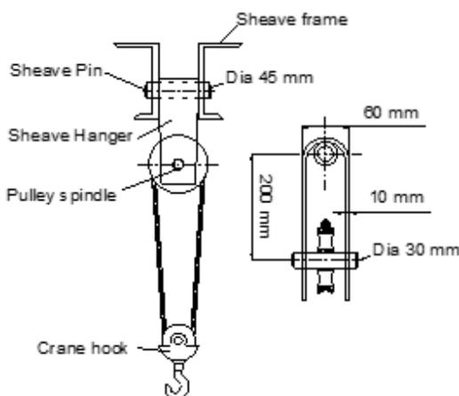
Fig. 1: The crane sheave assembly
