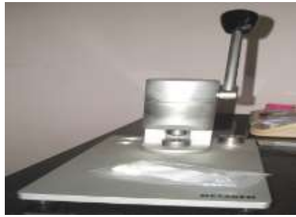
Fig. 6(b): Sealing press for crucibles
