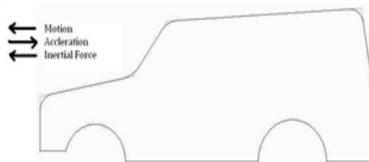
Fig. 2: Vehicle in Braking Mode:
