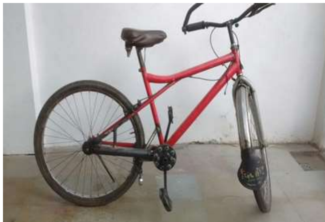
Fig. 1: Replacement of chain drive bicycle with driveshaft
