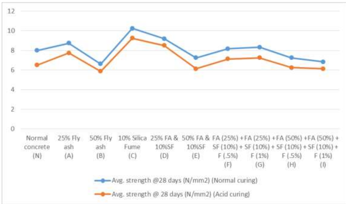
Fig. 9: Variation in strength by FTM in normal and acid curing.
