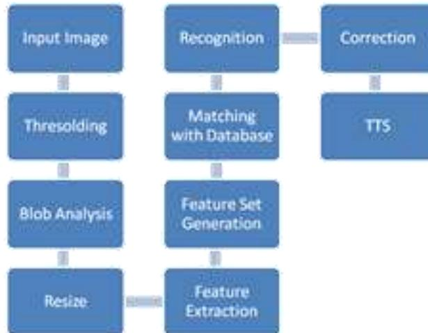
Fig. 1: Block diagram of OCR
