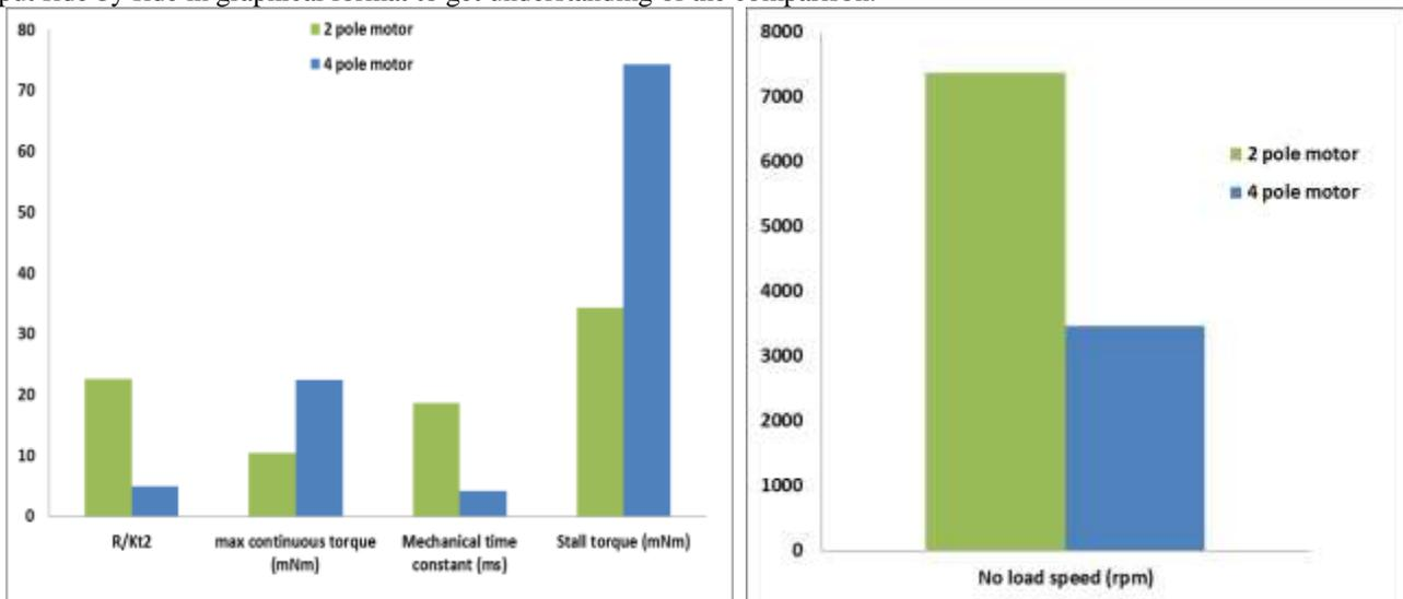
Fig. 4: Two pole vs four pole motor performance difference
