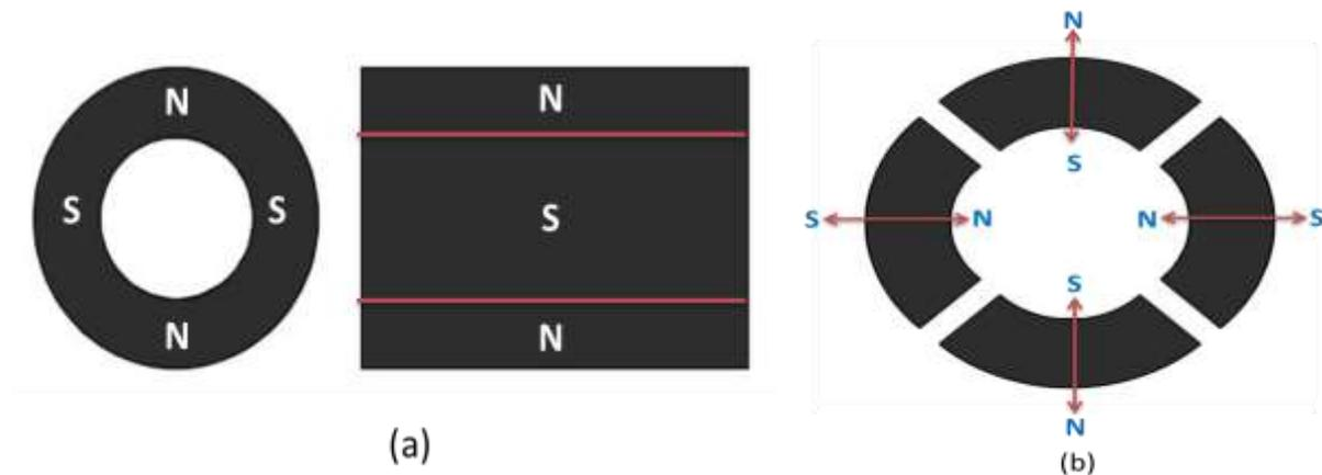
Fig. 3: (a) Isotropic magnet, (b) magnet tiles
