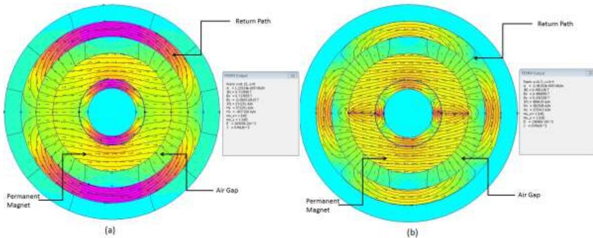
Fig. 2: (a) Two pole PMM 2-D FEMM, (b) four pole PMM 2-D FEMM
