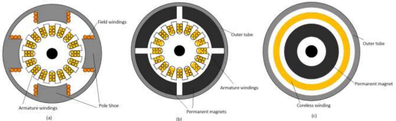
Fig. 1: (a) Conventional field wound motor, (b) Permanent magnet iron core motor, (c) Permanent magnet coreless motor
