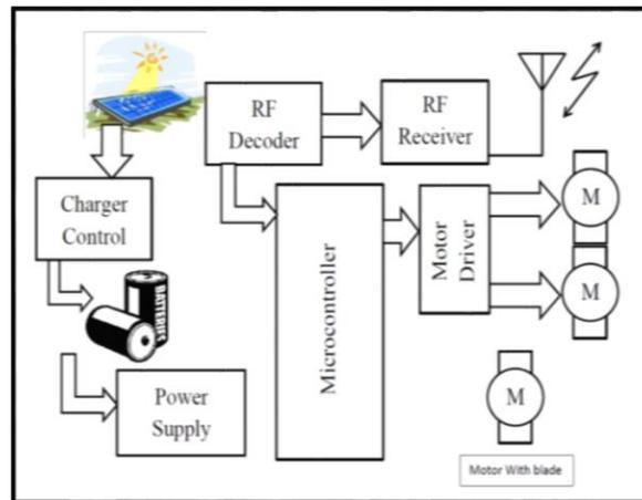
Fig. 1: Block diagram of Solar Based Wireless Grass Cutter
