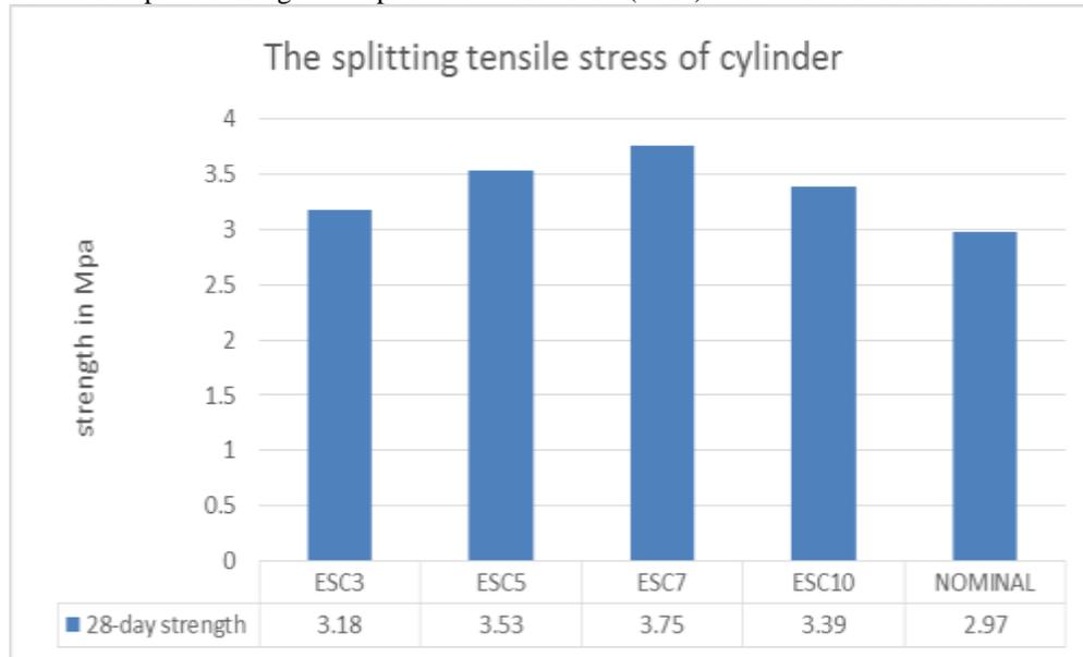
Fig. 3: Split Tensile Strength of Cylinder
