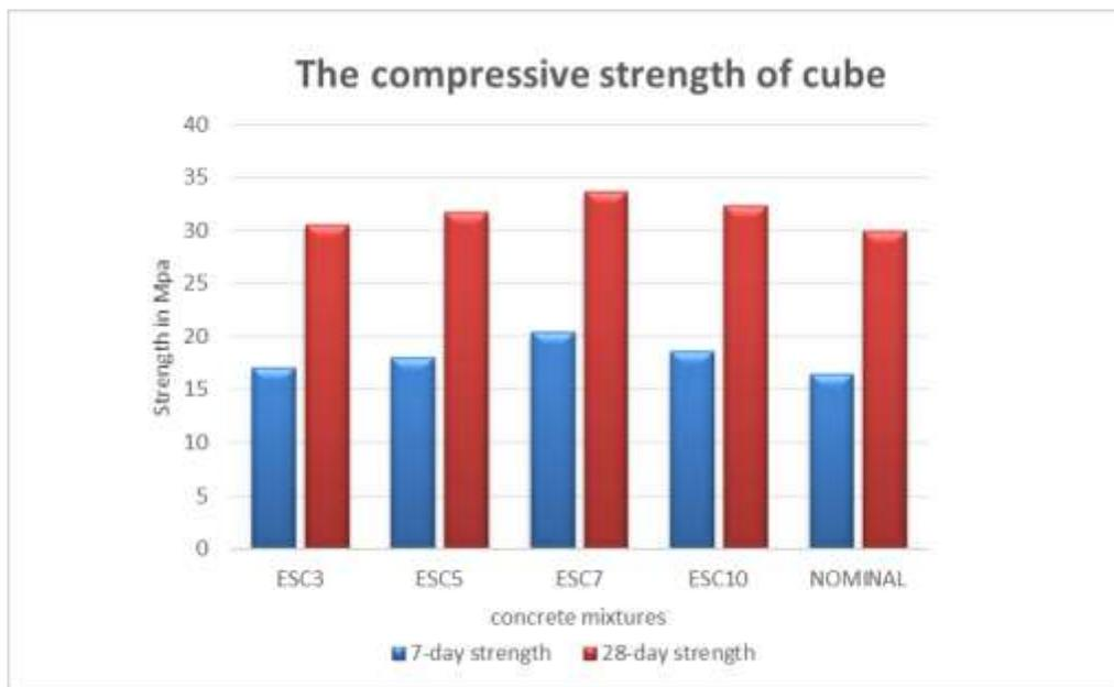
Fig. 1: Compressive Strength of Cubes
