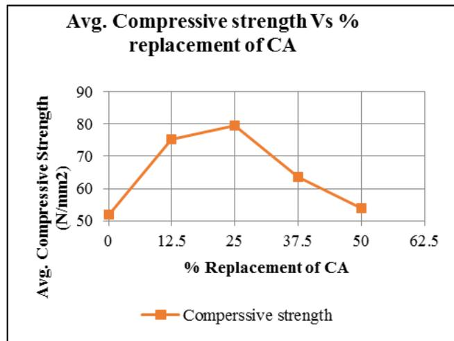
Fig. 4.1: Average Compressive strength Vs % replacement of CA
