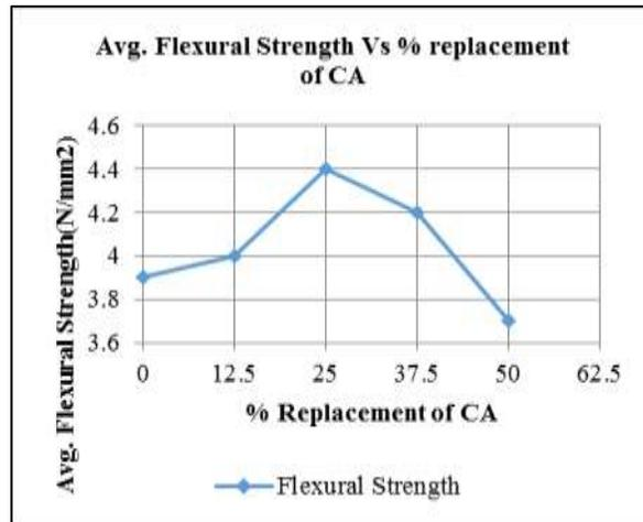
Fig. 4.3: Average flexural strength Vs % replacement of CA
