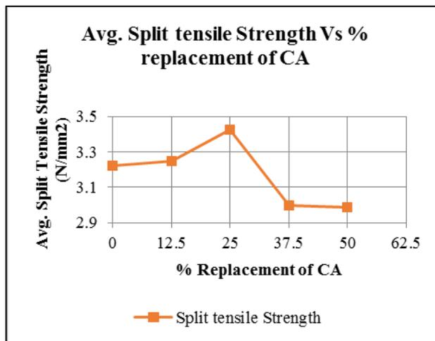
Fig. 4.2: Average split tensile strength Vs % replacement of CA
