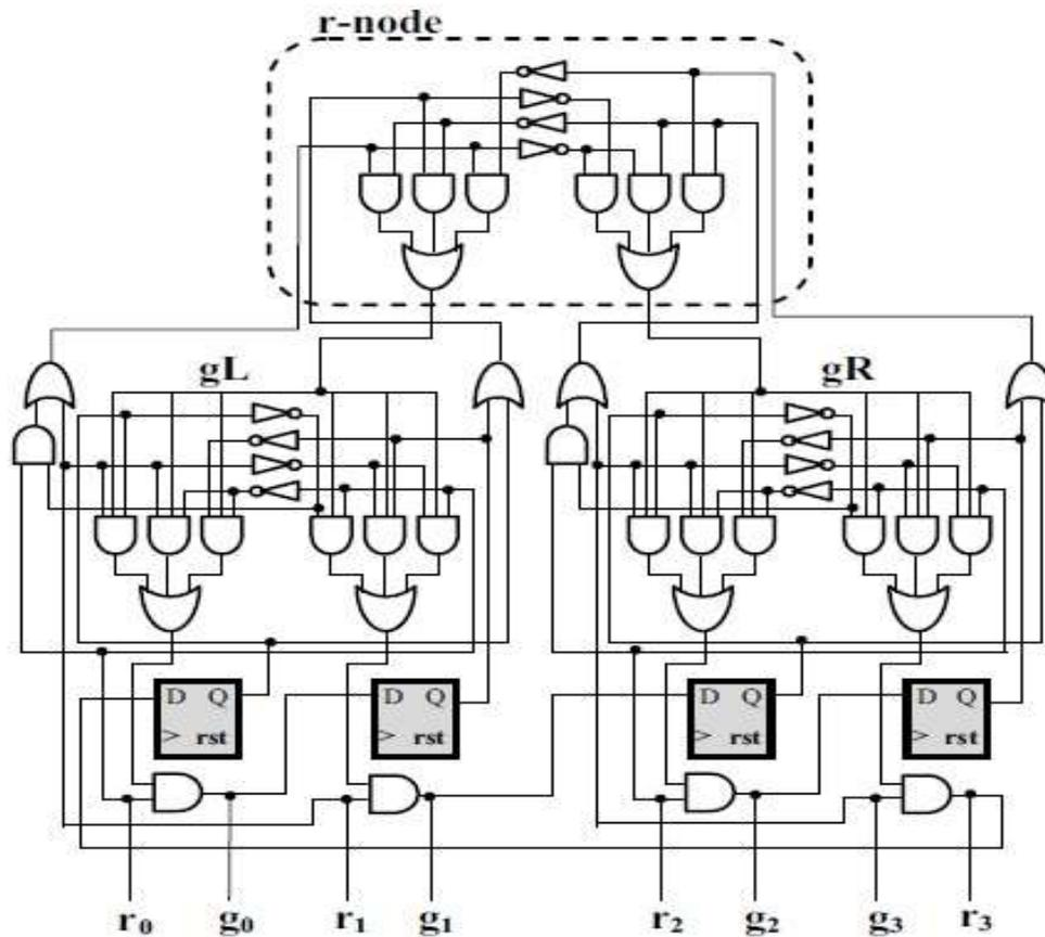
Fig. 3: 4- input PRRA architecture
