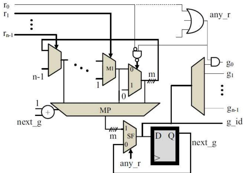
Fig. 5: Circuit of existing IRRA
