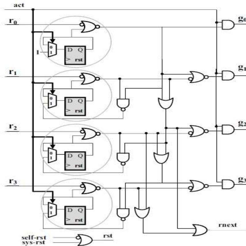
Fig. 4: 4-input HDRA architecture
