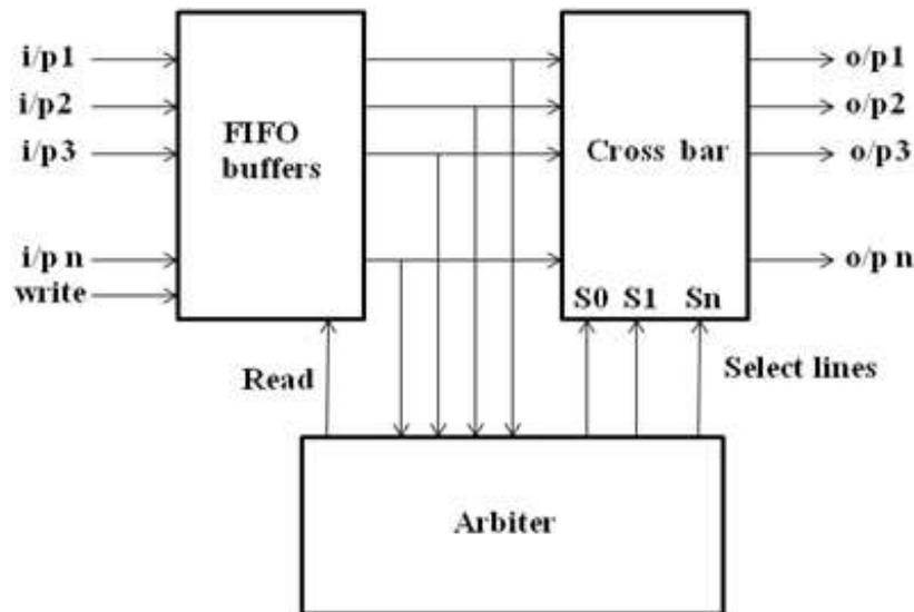
Fig. 2: Block diagram of NOC router
