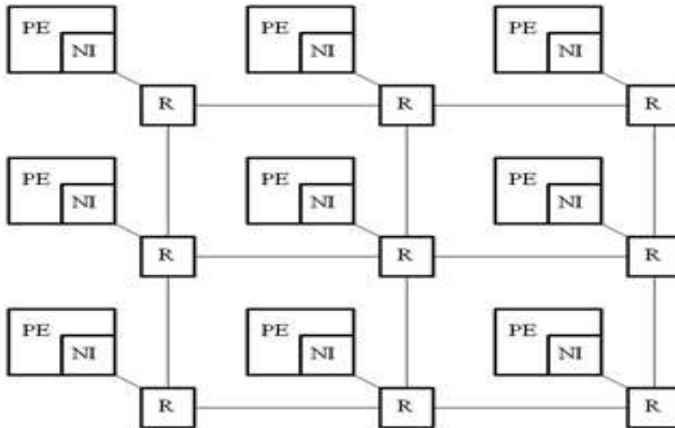
Fig. 1: Typical NOC architecture
