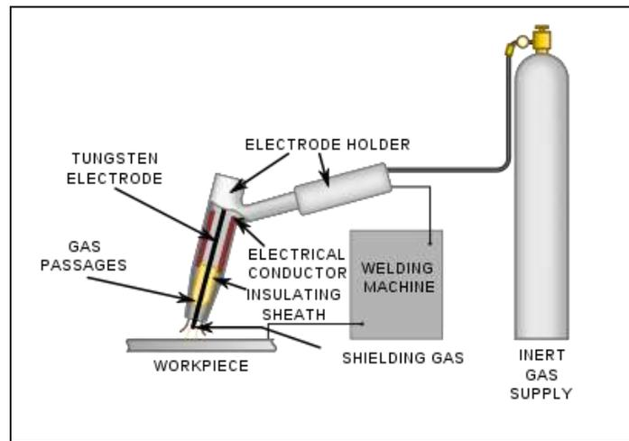
Fig. 3: Tungsten Arc Welding System set up
