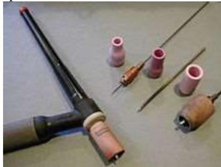
Fig. 1: GTAW torch with various electrodes, cups, collets and gas diffusers
