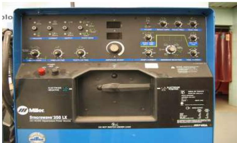
Fig. 2: Power Supply in TIG Welding
