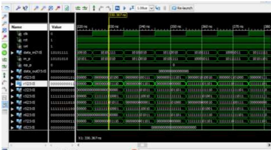
Fig. 5: Simulation result of FFT.
