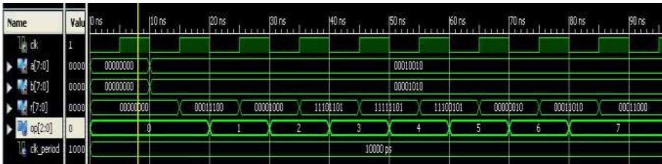
Fig. 4: simulation result of ALU operations.
