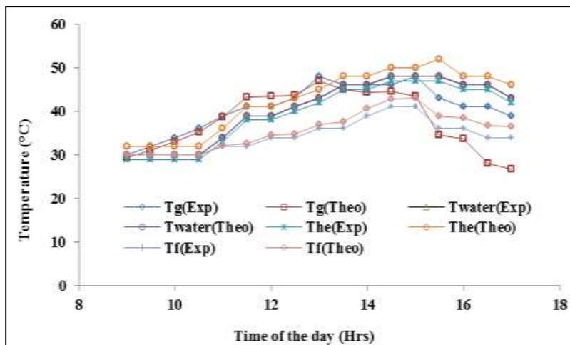
Fig. 2: Experimental and theoretical values of temperature elements of the pond.
