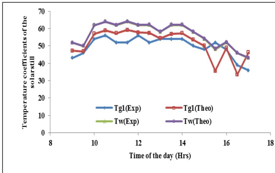
Fig. 7: Experimental and theoretical validation of temperature elements of the solarstill with multiple-wick materials.
