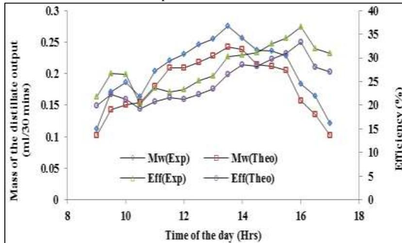
Fig. 4: Experimental and theoretical values of instantaneous distillate output and Efficiency of the solarstill with single wick
