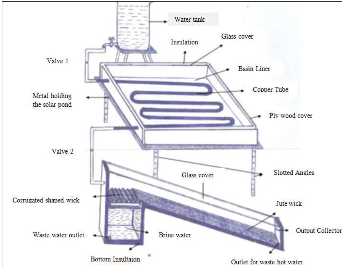
Fig. 1: Schematic representation of SSP and TWSS.
