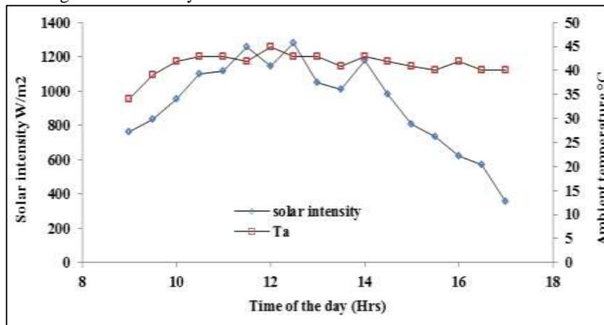
Fig. 5: Variations of solar radiation intensity and Ambient temperature with respect to time.
