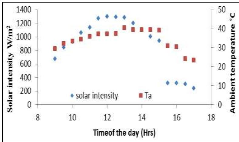
Fig. 1: Variations of solar intensity and Ambient temperature with respect to time.
