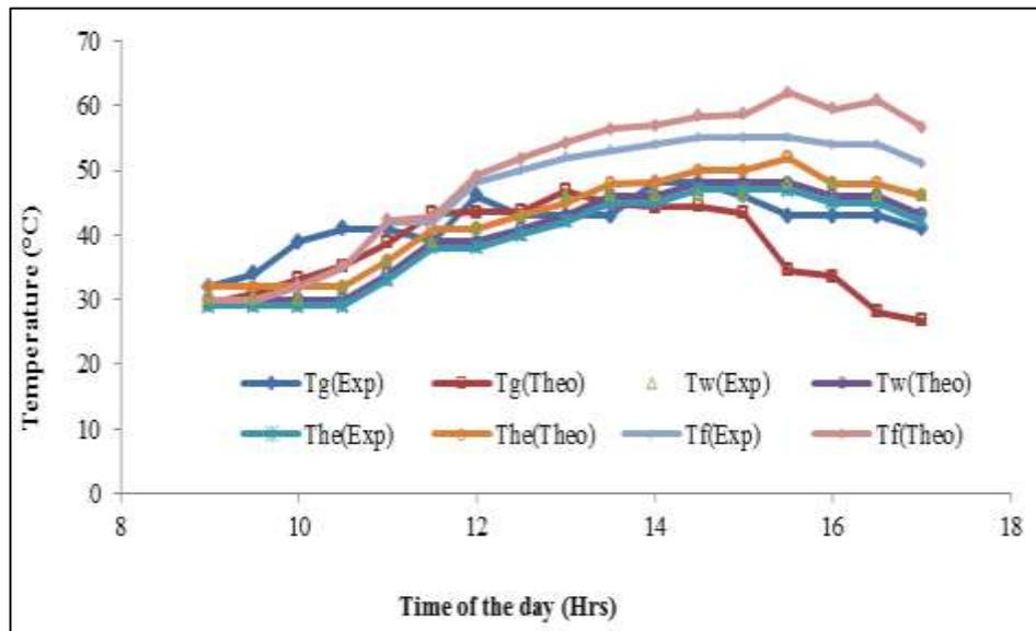
Fig. 6: Experimental and theoretical values of temperature elements of the pond.
