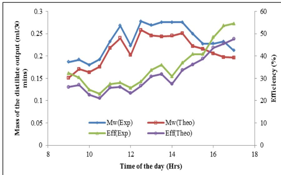
Fig. 8: Experimental and theoretical values of instantaneous distillate output and Efficiency of the solarstill with multiple-wick.
