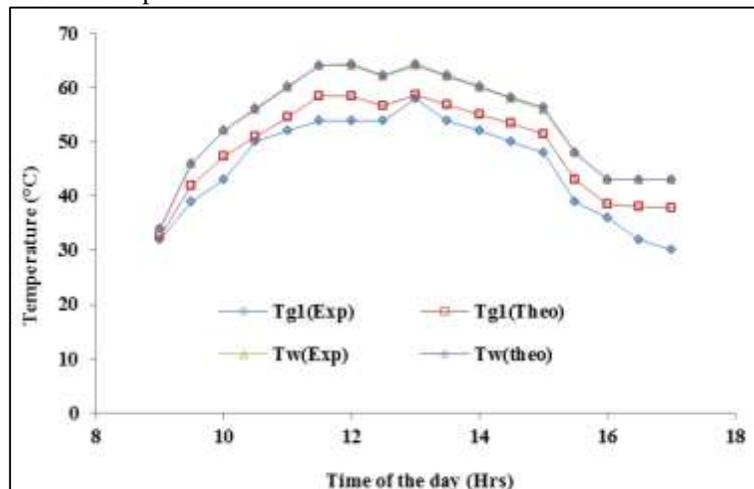
Fig. 3: Experimental and theoretical values of temperature elements of the solarstill with single wick material.
