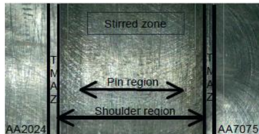
Fig. 9(a) FSW process carried using conventional milling machines with the aid of specially designed fixture Fig. 9(b): Macrograph of the welded sample
