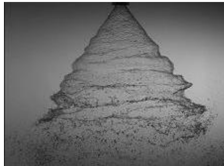
Fig. 1: Spray produce by pressure swirl atomizer.
