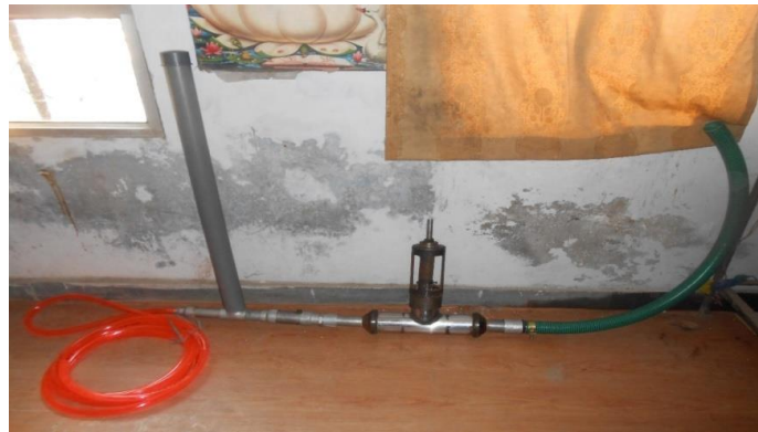
Fig. 2: Assembly of Hydraulic Ram Pump
