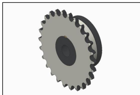
Fig. 3: 3D View of the Designed Sprockets with QD Bush Using Pro-E
