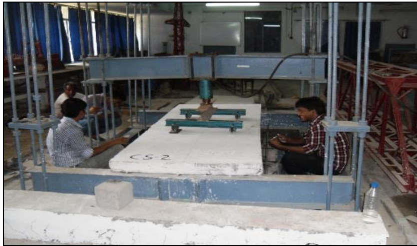
Fig. 4: Slab on Testing Frame
